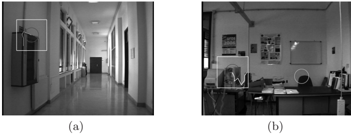
Fig. 6. a) The first landmark recognized by the robot. The red circle is the first fovea placing, while along the white line there are the subsequent movements. The large white square is the image region inside which fovea movements are allowed during the landmark memorization. b) The two landmarks detected in the lab near the corridor. The robot at first detected the salient point to the right, discarded it (see text) and memorized the second landmark to the left.
